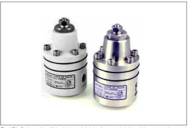
The LIR0x Series provide reliable shut down & isolation from control devices of the actuator whenever air pressure fails. If the supply air pressure drops below the mechanically adjusted set point (safety limit), the output line to the actuator (resp. both output lines with double acting) is sealed off. Rugged and corrosion-resistant – made of Aluminum alloy or in SS 316L. Compact small package size – light weight.
