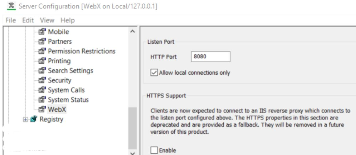
The IIS reverse proxy will offer HTTPS connections on port 443 by default, and optionally can be configured for HTTP connections.
