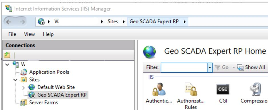
The IIS reverse proxy connects to the Geo SCADA Expert server's **Listen Port**. A revised set of properties are included for **WebX** settings in the Server Configuration Tool, in which you can set up the **Local Proxy** and **Network Proxy** settings. The **Network Proxy** is not usually required unless you have an additional proxy/firewall between the server and clients.
