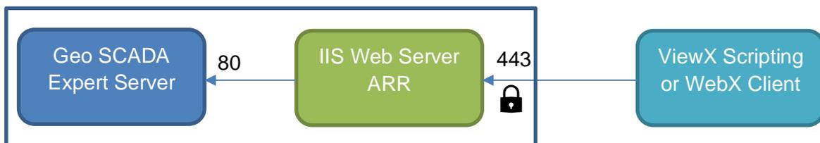
The IIS setup uses an Application Request Routing (ARR) module to direct web service calls to the Geo SCADA Expert server. The Geo SCADA Expert installation prerequisites include both IIS and ARR modules and set up a website:
