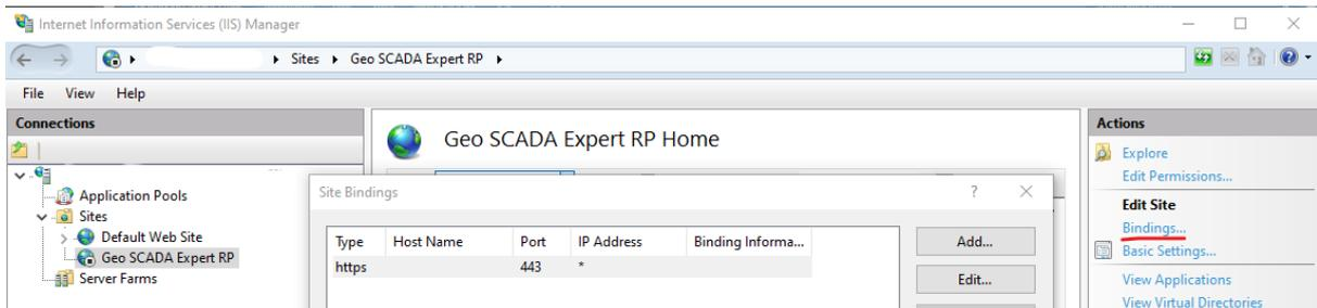
The Geo SCADA Expert server must be aware of the port(s) offered by the IIS server, and these are configurable in the **Local Proxy** section of the **WebX** page of the Server Configuration Tool (see in the help: 'Configuring Security and Connection Settings for Original WebX Clients' in the Guide to Security). This is required for ViewX to be advised of the web port(s) to be used for Mimic script access.
