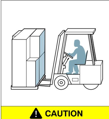
In order to lift the Flusarc 36 Unit, use a lift truck having an adequate lifting power with respect to the apparatus weight, by taking care to verify that the packing keeps perfectly balanced during the lifting phase.
