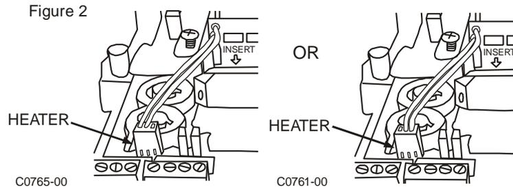
4. Connect the heater power supply wires as shown in Figure 3. If adding the heater kit to an existing installation, ensure that the power supply connected to the beam detector is adequately rated for the additional power consumption of the heater.
