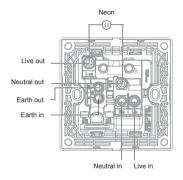
\* Neon indicator should be connected between Live Output and Neutral Output terminal.
