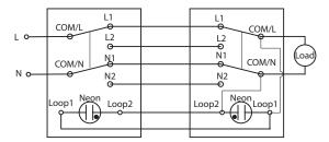
\* Customers have to connect the neon indicator with the circuit at the switch terminals.
