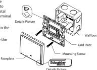
Insert a screwdriver into the clip lock, and twist the screwdriver to remove the faceplate.
