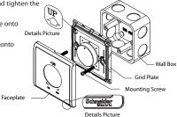
Insert a screwdriver into the clip lock, and twist the screwdriver to remove the faceplate.
