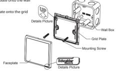
Insert a screwdriver into the clip lock, and twist the screwdriver to remove the faceplate.
