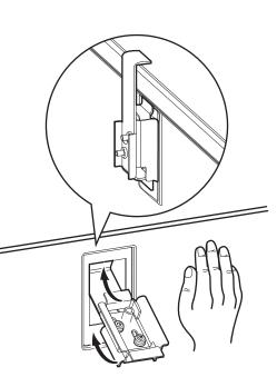
Secure the two screws in the lock assembly.
