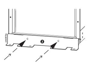
Push the PDU to slide the tabs on the bracket mounted to the PDU under the bracket bolted to the floor.
