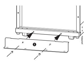
2 Secure the front anchoring bracket to the floor using floor anchoring bolts (not supplied). Use M12 strength class 8.8 or 1/2 inch, grade 5 steel bolts.
