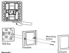
For surround mounting, align the clip locks on the faceplate and press firmly on the surround. Complete engagement of the clip lock is indicated by a clear "click" sound.
