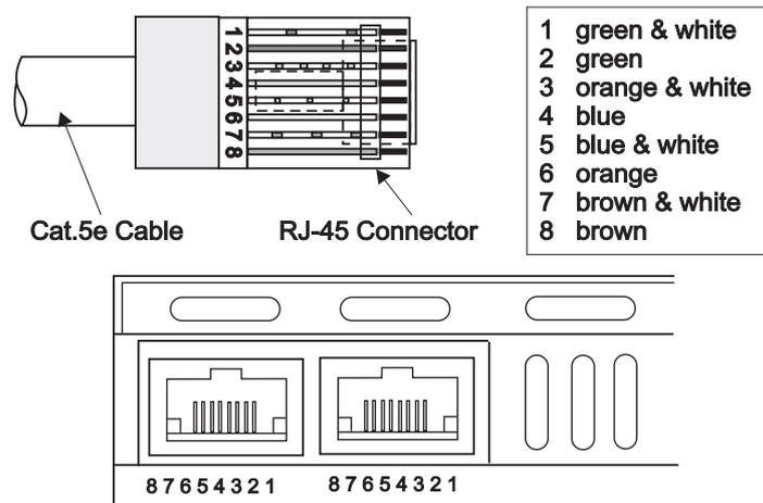
Figure 3. RJ45 pin assignments for plugs and sockets
