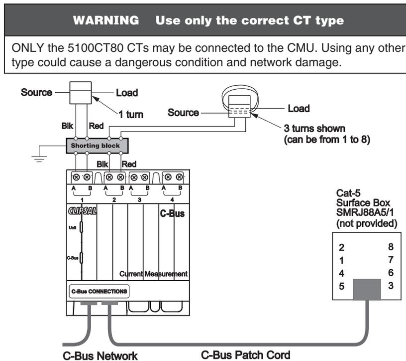
Figure 1. Wiring diagram
