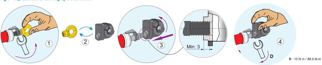
Fig.6 Setting with the cable tensioner
