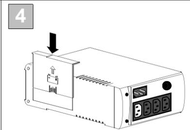
Align the battery compartment cover with the grooves in the UPS. Slide the cover down until it locks.
