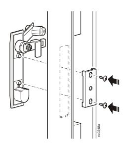
**To replace the cam:** If you have a NetShelter VX enclosure, replace the pre-installed NetShelter SX cam with the NetShelter VX cam (provided).
