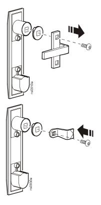
**To reverse the door handle:** If you reverse the door, complete the following steps to properly orient the door handle:
