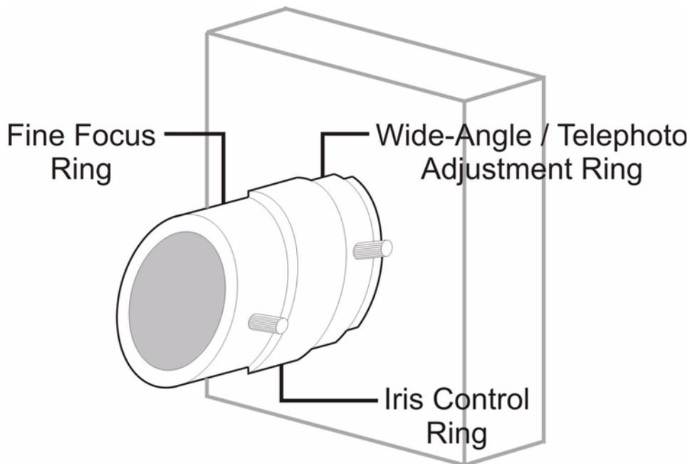
Note that the Wide-Angle / Telephoto Adjustment Ring and Fine Focus rings each feature a locking screw. These screws will be used to lock the rings in place once you are satisfied with your focus settings. Once they are locked in place these locking screws prevent the focus rings from turning due to manual interference or vibrations, thereby ensuring that additional focus adjustments will not be necessary.
