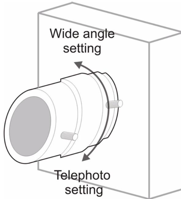
5. Loosen (but do not completely unscrew and remove) the locking screw on the Fine Focus Ring. Then, while referring to the image that is displayed in the Basic or Advanced View, make small adjustments to the position of the Fine Focus Ring until you are satisfied with the image that is displayed in the Basic or Advanced View. Then, tighten the locking screws on the Fine Focus Ring and the Wide-Angle / Telephoto Adjustment Ring to lock them in place.
