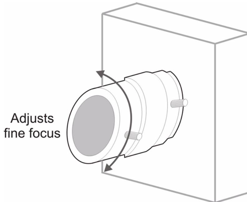
**Note:** If you are unable to get the image into focus you may need to readjust the Wide-Angle / Telephoto Adjustment Ring, then try adjusting the Fine Focus ring again.
