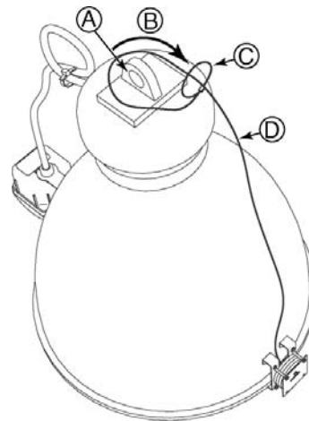
Figure 3: Loop the Safety Wire around the Mounting Stem
