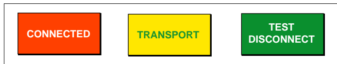
Figure 4: Circuit Breaker Position Indicator Flags
