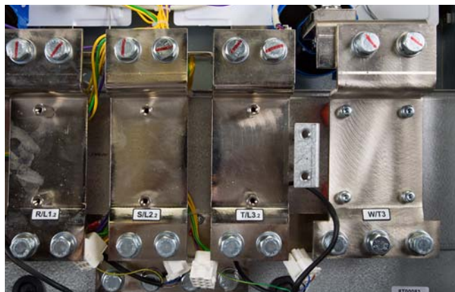
Figure 116: R/L1.2, S/L2.2, T/L3.2 Bus Bars
