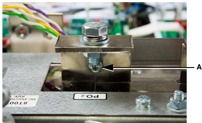
Figure 37: Bus Bar Connection Detail
