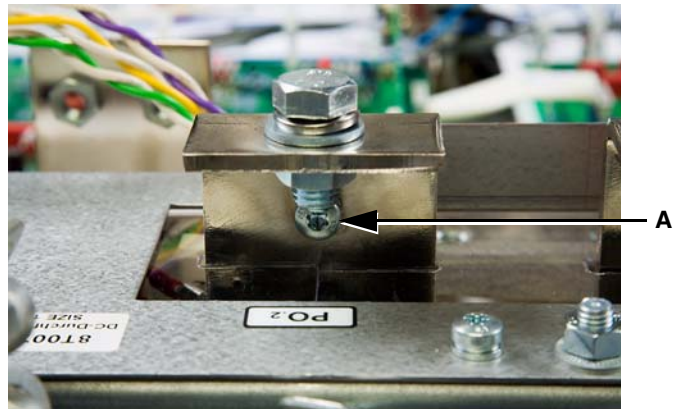
Figure 136: Top Terminal Bracket Mounting Hardware
