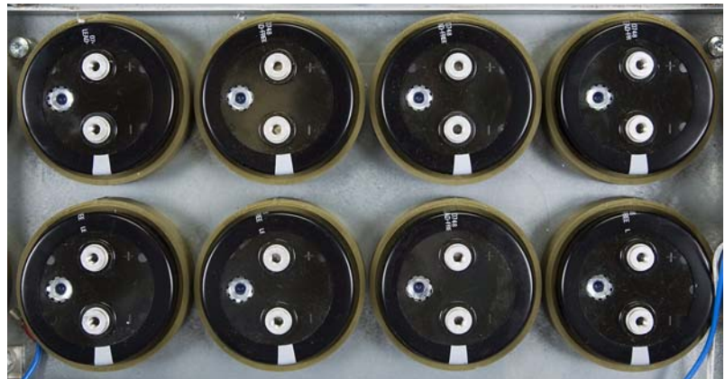
Figure 133: Capacitors, Phase V Shown
