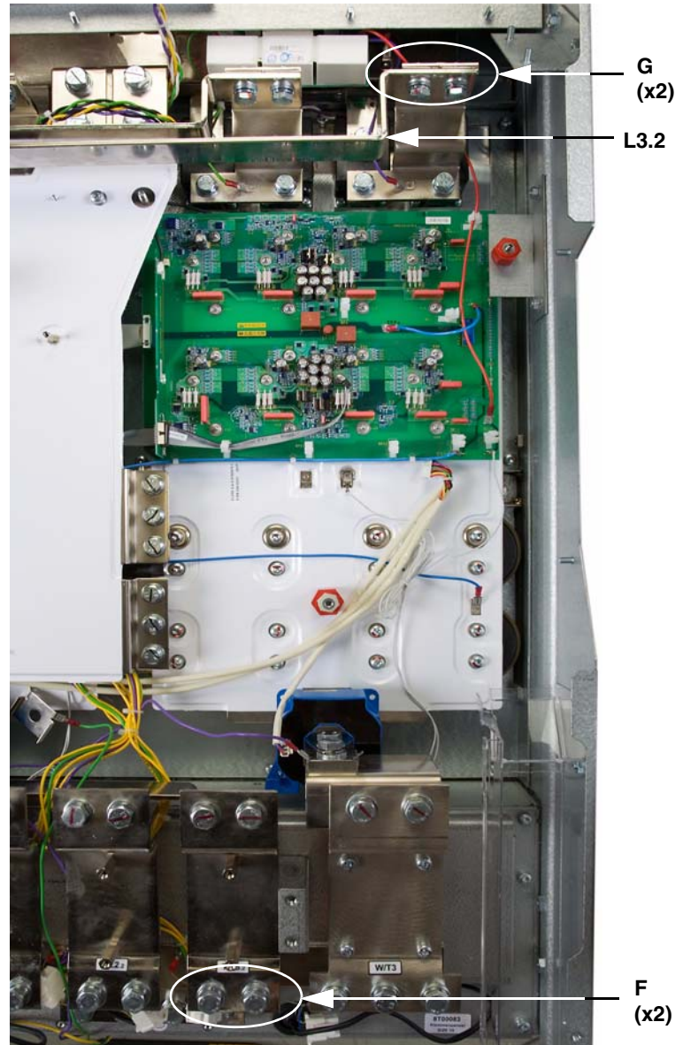
Figure 176: L3.2 Input Bus Bar
