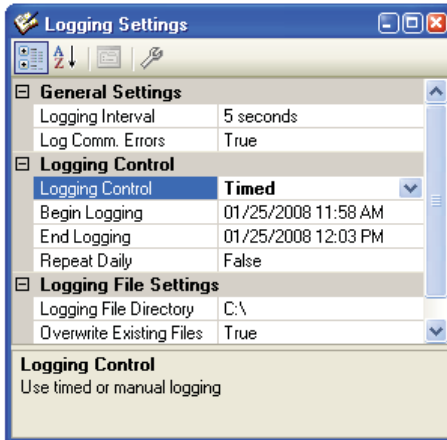
Figure 19: Logging Setting Window with Timed Logging Enabled
