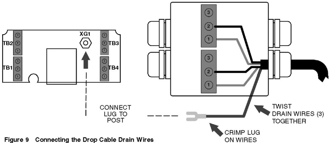
Figure 9 Connecting the Drop Cable Drain Wires
