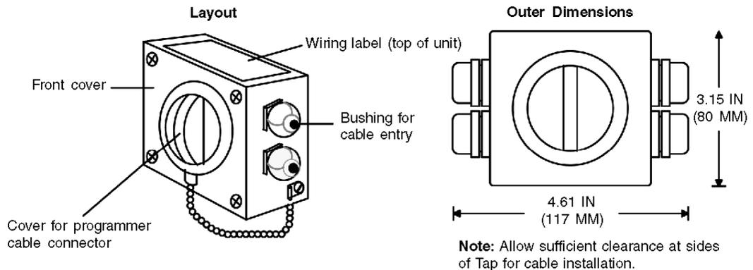
**Figure 1** Dimensions and Clearances
