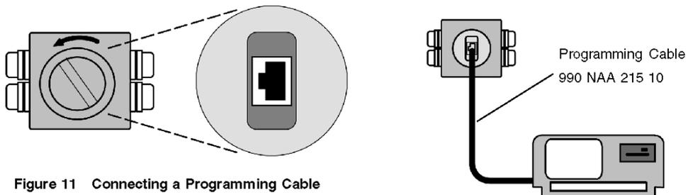
**Figure 11 Connecting a Programming Cable**
