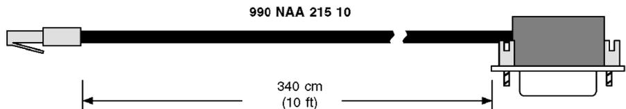
**Figure 12 Detail: Programming Cable (990 NAA 215 10)**
