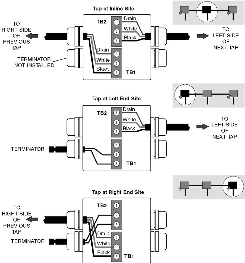
Figure 7 Connecting the Trunk Cable Wires and Terminator
