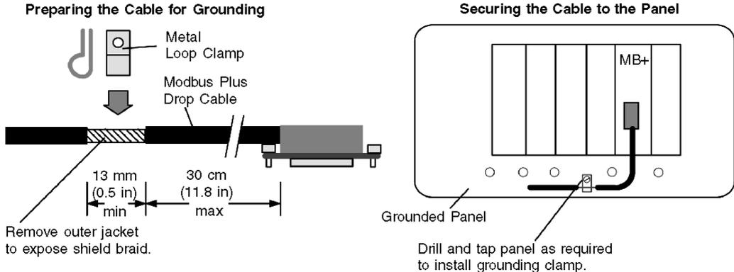
Figure 10 Grounding the Drop Cable at the Device Panel
