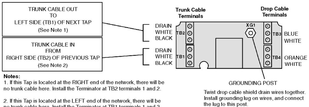
**Figure 4** Wiring Terminal Locations
