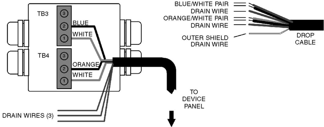
Figure 8 Connecting the Drop Cable Signal Wires
