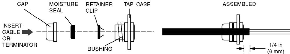
Figure 5 Method of Insertion into Tap Bushings
