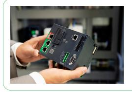
The new IIoT-ready Modicon M262 controller provides cybersecure connectivity, data management and visibility to remote machines. Designed and shipped with embedded cloud connectivity, the M262 enables machine builders to securely manage both equipment efficiency and predictive maintenance, without having to send engineers to remote end user sites.
