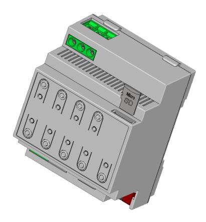
After the label has been removed, carefully insert the SD card into the disconnected gateway in such a way that the row of contacts points downwards and the recess in the card points towards the left. Please make sure to insert the card straight into the slot without any angle or bend. You will notice a slight pressure when the contact row has snapped into place.
