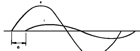
FIGURE 12 TYPICAL WAVE FORM SHOWING LAGGING CURRENT
