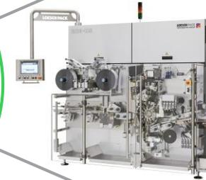
The automation solution for **Norden's** tube filler is based on PacDrive 3 to control the complete machine with a single controller platform.
