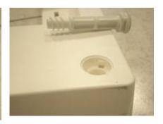
11) Take the base and remove the rail din block:
