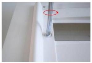
3) Remove the screws from the plastron with a strong hit:
