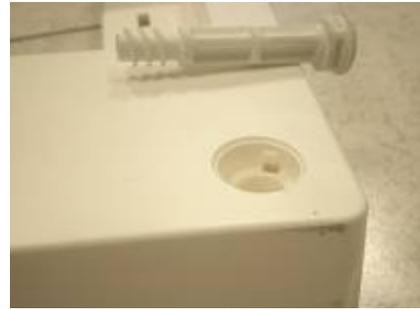
11) Take the base and remove the rail din block:
