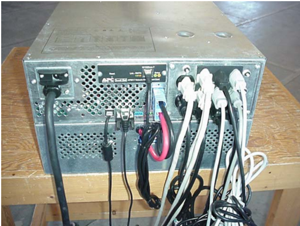
Configuration for Radiated Emissions (Rear Close-up)
