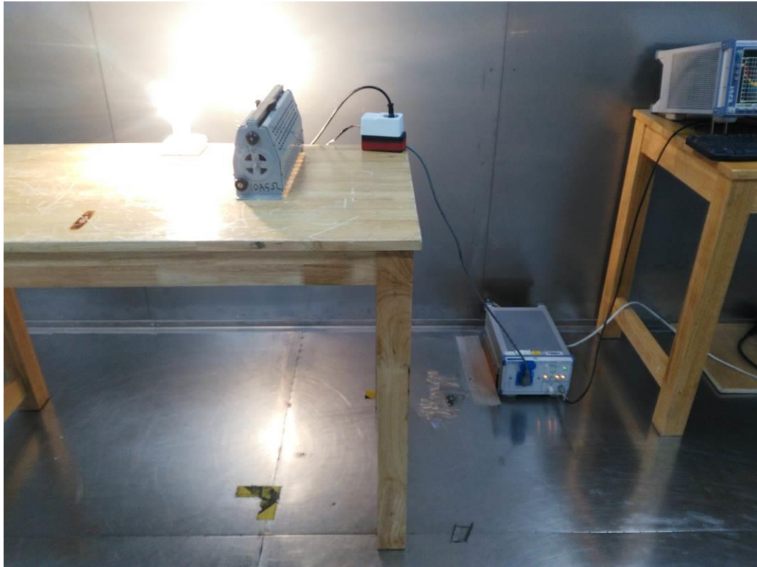
Figure 2 Mains conducted disturbance voltage test setup
