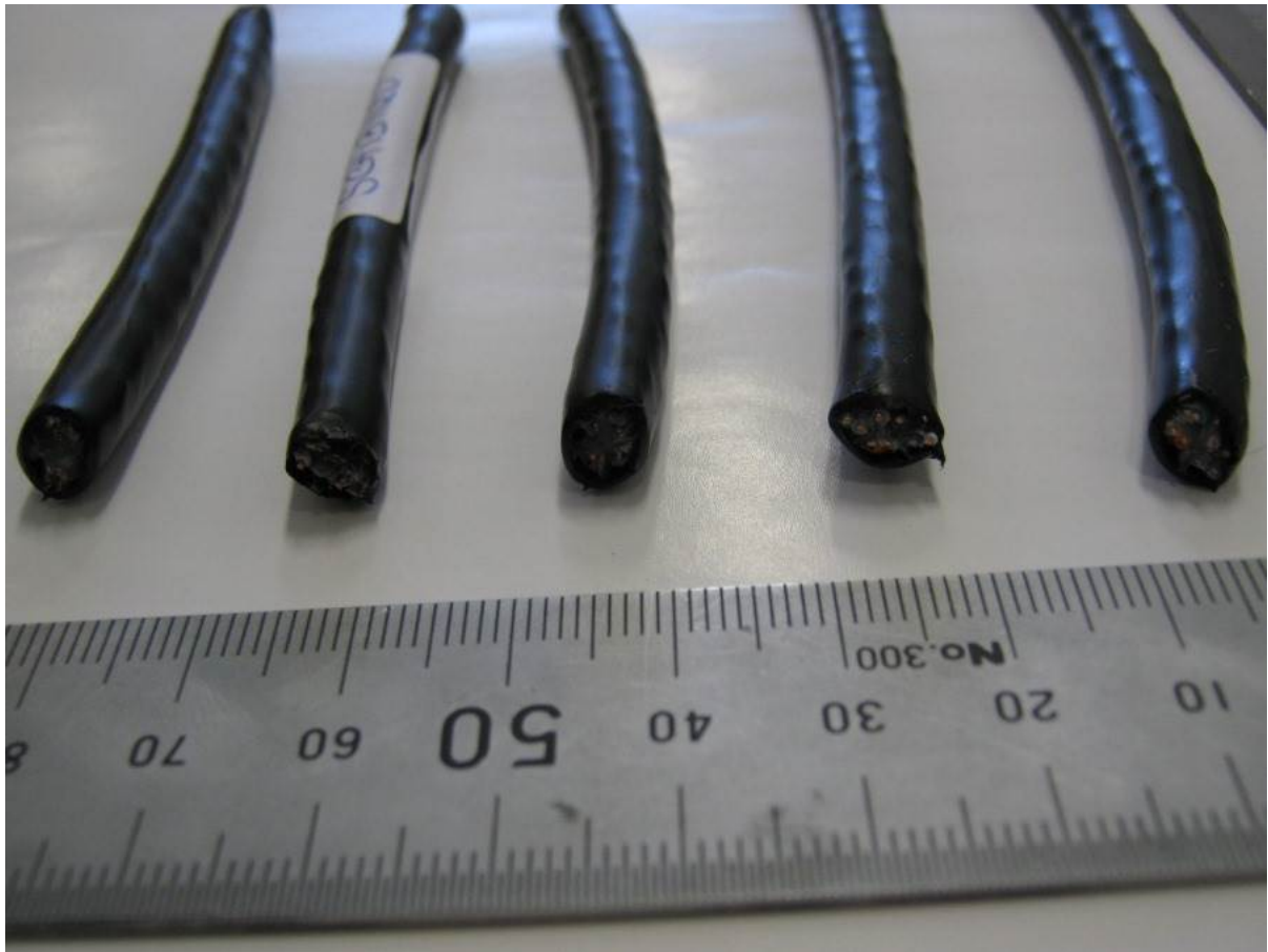
Fig. 1.b. Samples before test with dimensions – side view from cable ends
