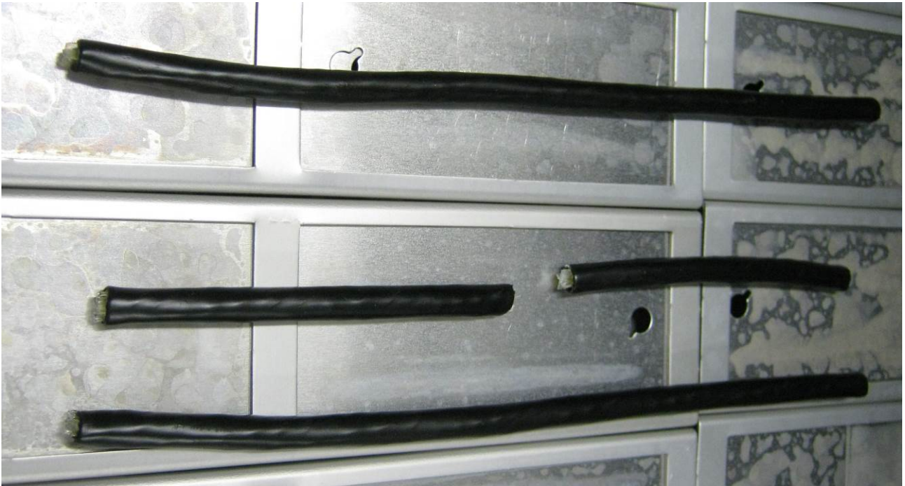
Figure 3.a. Samples after 360 hours of radiation – inside test chamber
