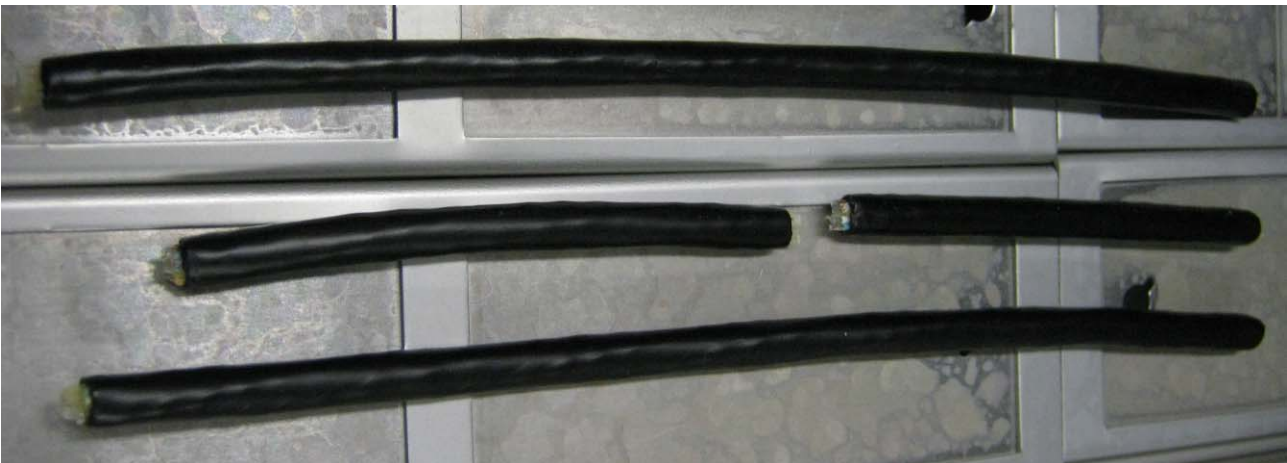
Figure 3.d. Samples after 864 hours of radiation – inside test chamber
