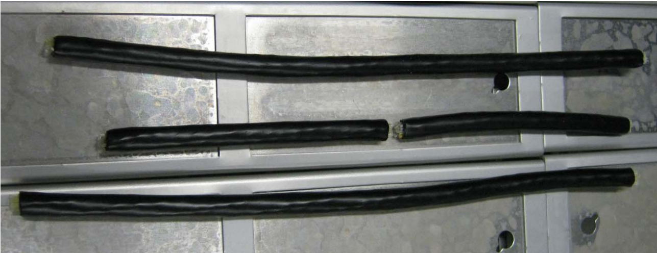
Figure 3.c. Samples after 696 hours of radiation – inside test chamber
