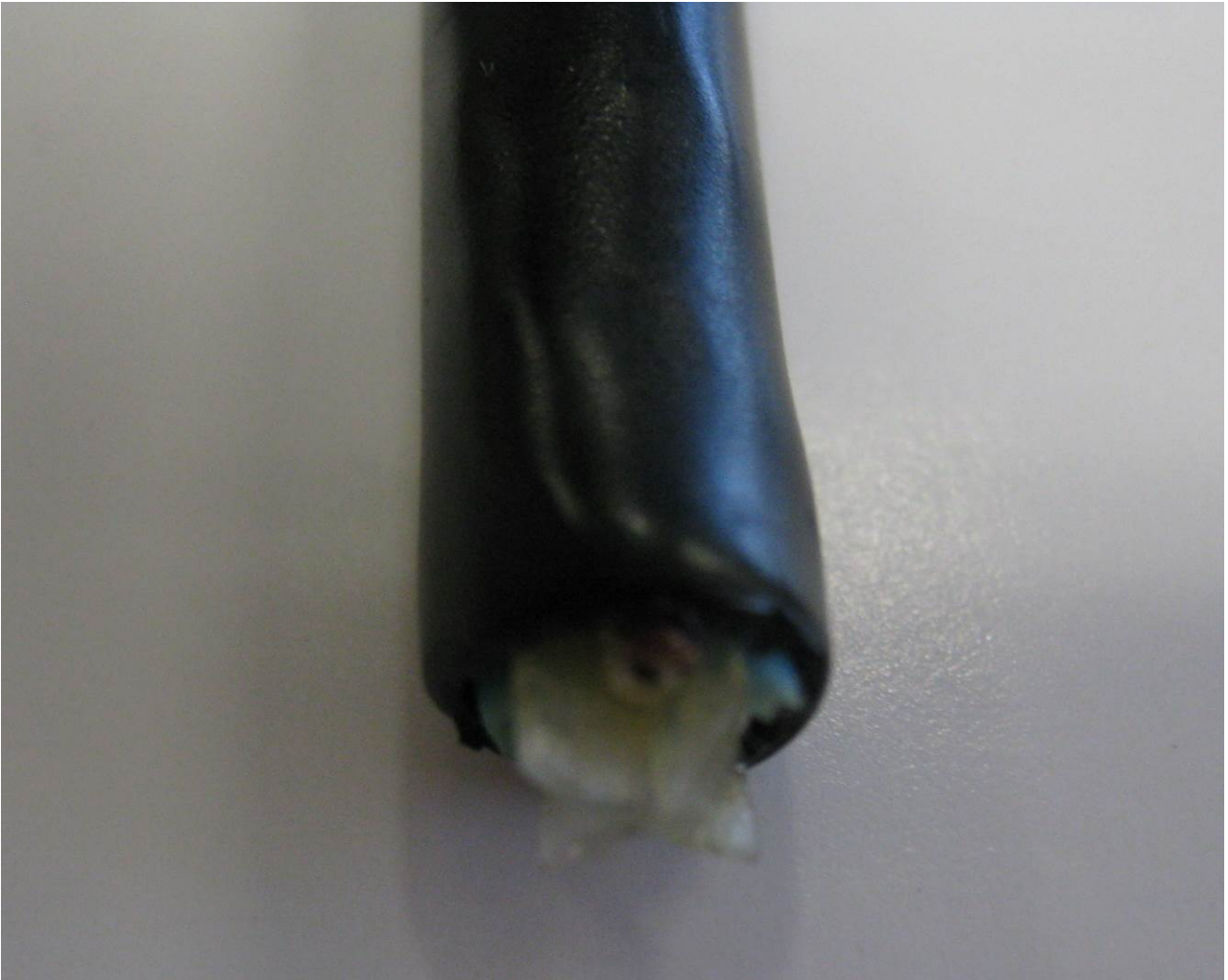
Fig. 2.d. Retracted sheath at cable end, after 960 hours of radiation
