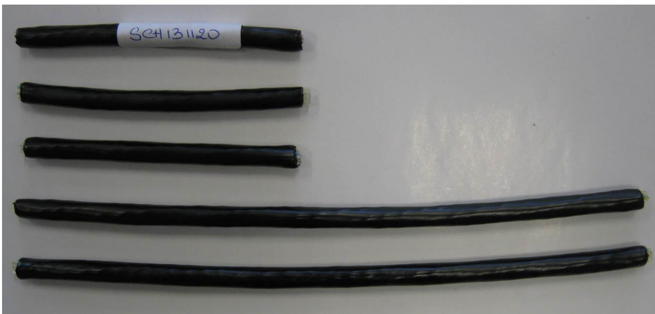
Fig. 2.b. Samples after 960 hours of radiation – top view (The top sample with label was not radiated)
