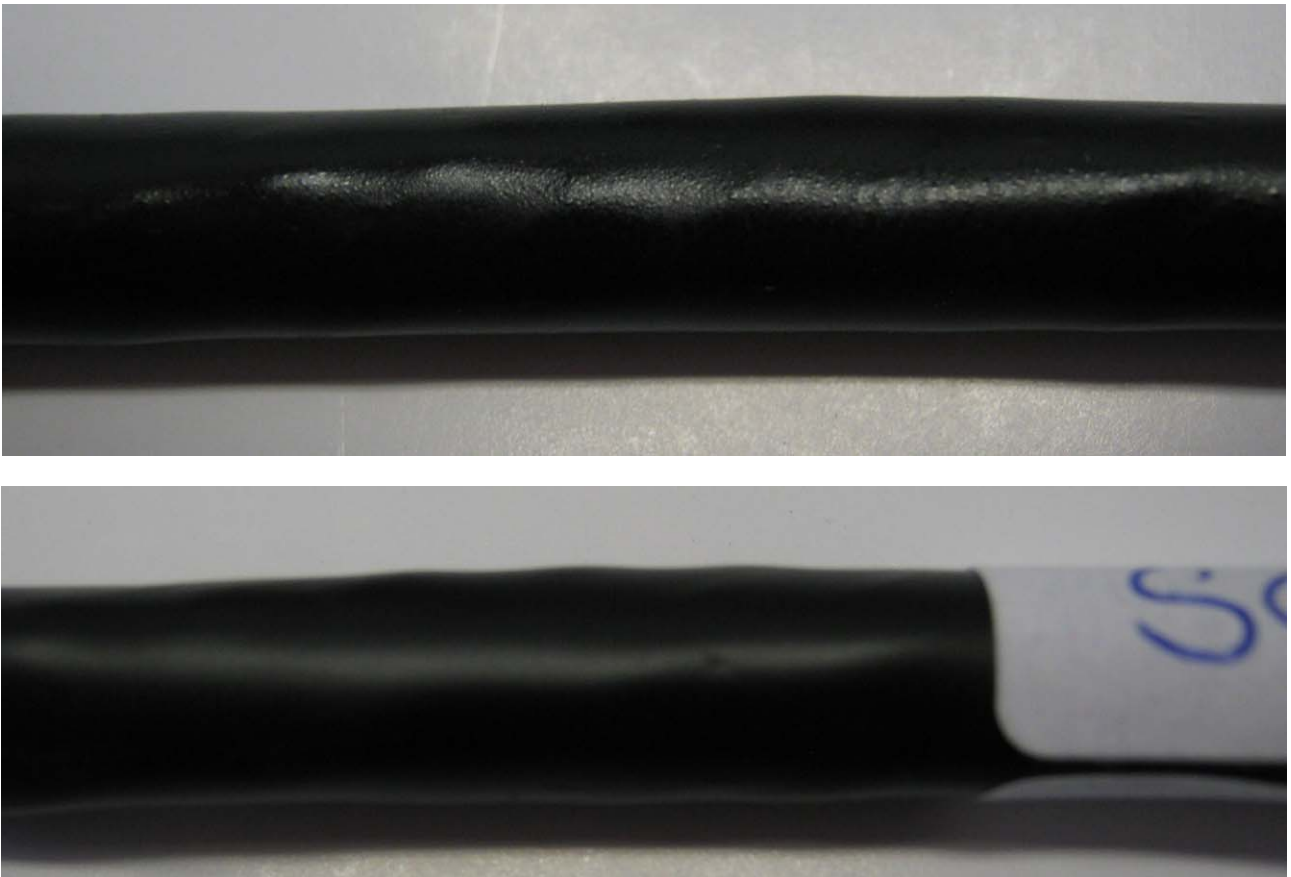
Fig. 2.e. Surface of 960-hour radiated sample (top) compared to non-radiated sample (bottom)
