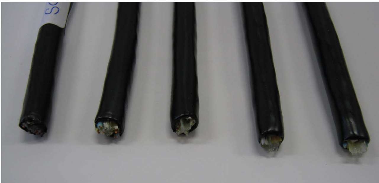
Fig. 2.c. Samples after 960 hours of radiation – side view from cable end (The left sample with label was not radiated)
