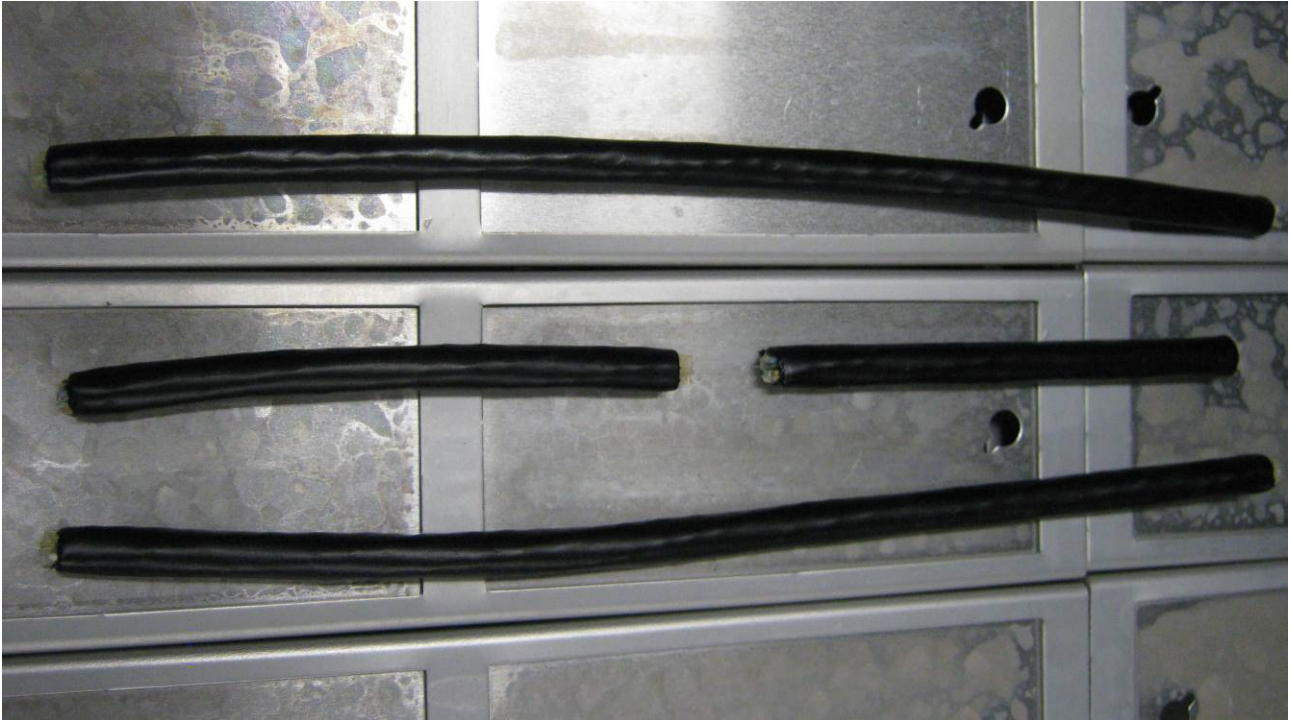
Fig. 2.a. Samples inside the test chamber after 960 hours of radiation
