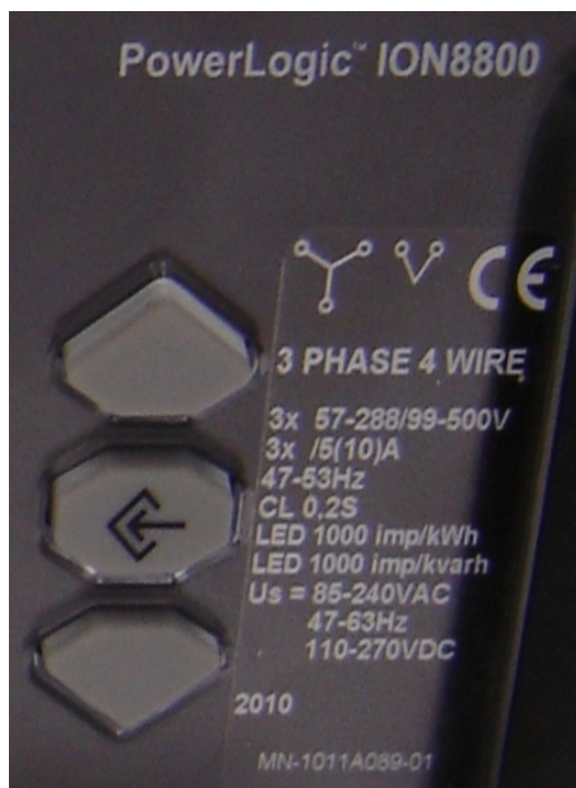
Schneider Electric Model PowerLogic ION 8800 Electricity Meter (including sample markings)
