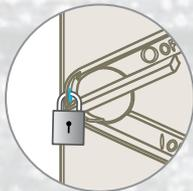
Lever is lockable in the off position for greater safety and no electricity during maintenance
