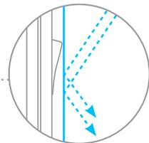
UV-impervious membrane filters out UV and protects the switch from damage caused by sunlight
