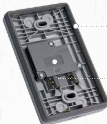
Co-injection moulded gasket on the base plate seals tight with the cover plate, avoiding any penetration of water and is more durable than the conventional O-ring design
