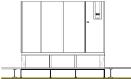
Unit with fan plenum installed above the raised floor
