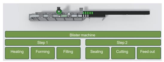
Equipment Modules add a standardized interface and behavior for command processing, operation modes, exception handling, and logging – on top of the functionality provided by AFBs. EMs consist of one or more combined AFBs. Equipment Modules for typical machine parts include: Axis Module (combining AFBs for homing, jogging, endless, positioning, and cam functions), Crank, Multibelt, Robotic, Smart Infeed, Unwinder, and Intelligent Line Shaft.
