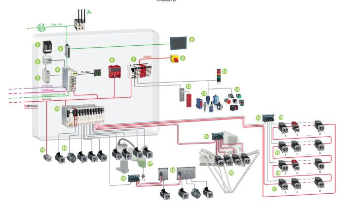
**Synchronized axes & robots / Sercos / Motion controller PacDrive LMC802** for higher requirements
