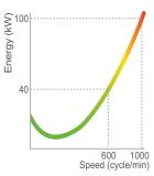
Measure the energy consumption of a running machine compared to the output and calculate the optimal ratio
