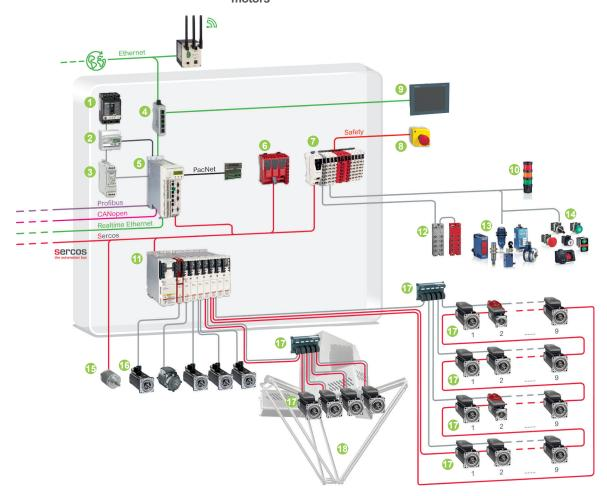
Synchronized axes & robots / Sercos / Motion controller PacDrive LMC802 for higher requirements
