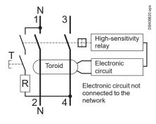
The toroid provides information on the leakage current and the power required to trip the device.
