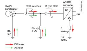
The DC leakage current generated by the DC voltage source and produced by the AC/DC converter (DC bus) only flows through the RCDs connected in parallel in the event of an insulation fault in a parallel load or in the event of contact with the parallel outgoer.
