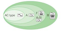
The increase in use of electronic loads can result in earth leakage current with different waveform characteristics. This situation must be carefully analyzed as it affects the performance of RCD. That is why the IEC series of standards has defined four types of RCD.
