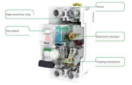
The residual current device consists of:
