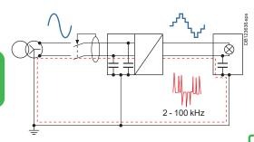
Rule 1: use a Schneider Electric A-SI type residual current device
