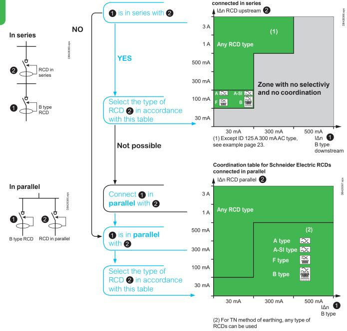
If more than one B type RCD is connected in series and in parallel in the installation, the RCD 2 shall be in accordance with Selector no. 7
