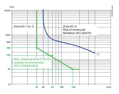
■ The IEC 60479 international standard studies the sensitivity of the human body to the electric current. Curve C1 defines for each current value the maximum time before a person is at risk of ventricular fibrillation.
