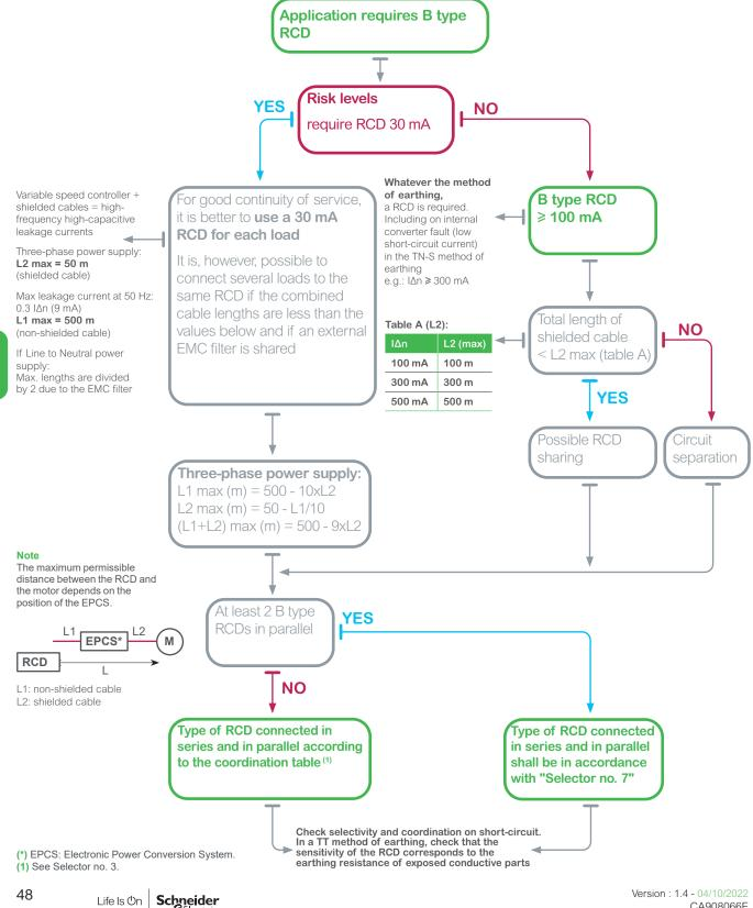
If many converters, EMC filter must be mutualized and each internal filter must be disconnected to limit leakage current.
