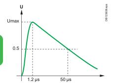
Fig. 2: normalized voltage waveform 1.2/50 µs
