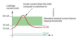
The estimated continuous leakage current of a computer is approximately 2 mA. This leakage current is very weak and therefore not dangerous.
