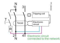
In the case of VDT technology ("Voltage Dependent Technology"), the toroid only provides information about the leakage current. The power required for tripping is supplied by the electrical network.
