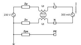
In this case measurement current pass through the 2 RCD windings in opposite polarity and the total Self L = Lt - Lt ~0. (magnetic leakage is negligible).
