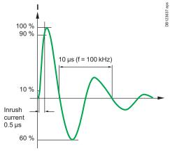
Fig. 3: normalized current waveform 0.5 µs/100 kHz
