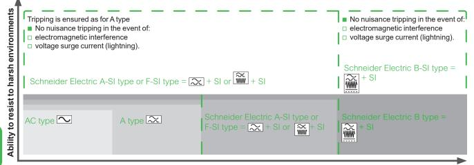
Ability to detect earth leakage depending on the type of load in accordance with the IEC series of standards
