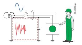
As RCDs are designed to detect very low currents (e.g.: 30 mA), interference due to the network or its environment can, in certain cases, result in RCD tripping. Nuisance tripping is disconnection of the power supply when no hazardous situation exists. This type of tripping is often repetitive, which is highly detrimental to the quality of the electricity supply and causes operational interference for the user.
