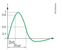
Fig. 4: normalized current waveform 8/20 µs
