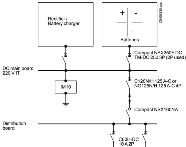
**Table C.1: circuit breaker selection for 220 V DC according to earthing system**
