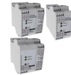
4AO/8SW/4AO-8SW – Analog and Discrete Output Modules
