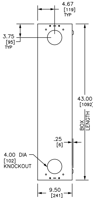
TYPICAL BOX SIDE VIEW
