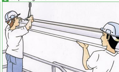
3 Suspending the Canalis KBX on cables
