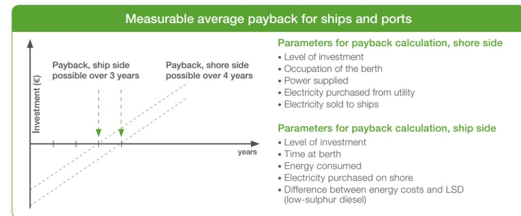
(7) Based on 11 stopovers per year, 72 hours per stopover, average consumption of 1.6 MW
