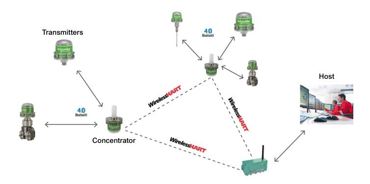
Hybrid architecture using WirelessHART mesh networking coupled with ultra-efficient BLE Instrument Area Networks
