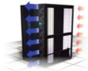
Rack air containment
