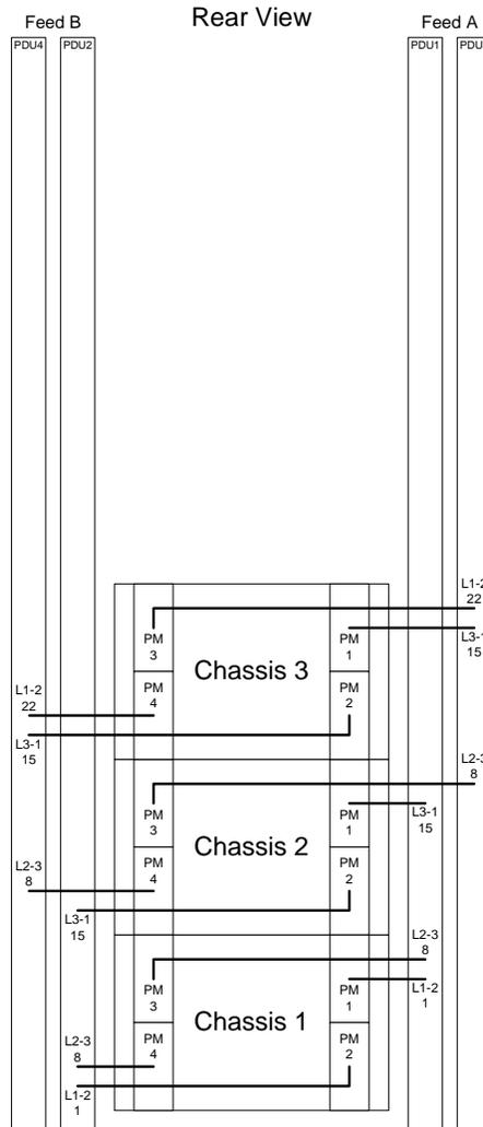
Note: Outlet numbers shown are for power supplies with C20 inlets. If using power supplies with C14 inlets, add 1 to the outlet numbers above.
