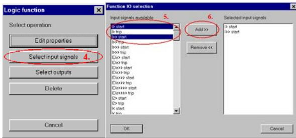
On this example we are making a function block which output is used as a common overcurrent alarm signal for Profibus. Select the required start signals from the left list and then press the 'Add' button. Press 'OK' when finished.
