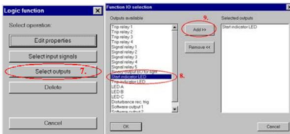
On this example the logic output is only used by Profibus, thus the function output is connected just to an alarm led. At least one output connection is required, even if there are no other purposes for the output than reading from the bus.
