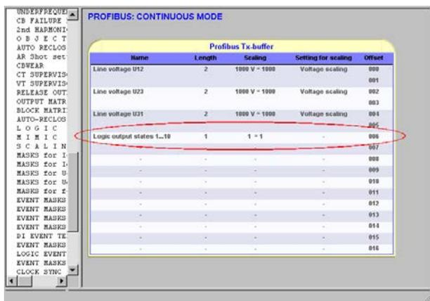
Add the logic outputs to appropriate offset by left clicking a line, and selecting 'Logic Outputs' from the appearing 55list.
