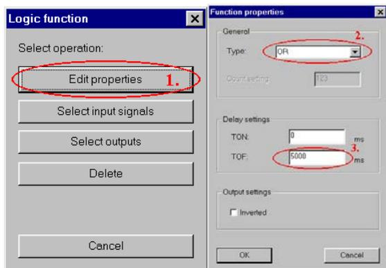
Change the function type to 'OR'. Protection signals operates very fast, thus a release delay is needed for keeping the signal active a sufficient time. Otherwise Profibus master can miss rapid signal changes. The delay should be set to a value of 500 ms or greater, depending on how often master polls the slave. Press 'OK' when finished.
