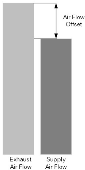
Figure_5: Negatively pressured room
