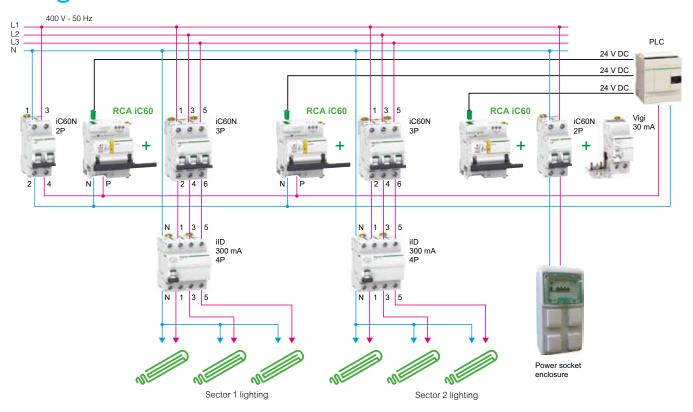
Note: to insure closing of neutral before phases the control of lightings must be realized by RCA and not by iID.
