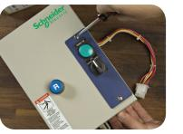
Plug Instakits into the terminal block and put the cover in place.
