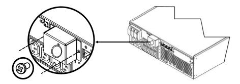
4. Run #10 AWG gauge (5 mm<sup>2</sup>) wire through the access panel, and connect the wires to the terminal block (green: ground, brown: hot, blue: neutral). Use an appropriate strain relief (not included).
