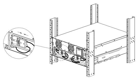
**3** Secure the battery connectors with 8 (M3x18) screws.
