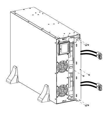
Connect battery input wires.
