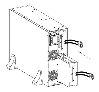
Secure the battery compartment door of the battery pack.
