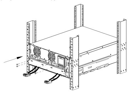
**②** Connect battery input wires.
