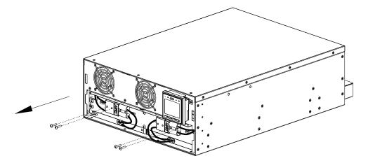
4 Disconnect UPS battery input wires.
