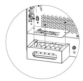
2 Pass the input and output wires through the opening in the housing. The output ground wire is connected to the outer shell.
