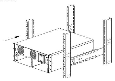
**9** Secure brackets to the pillar of Rack by 4 (M5x12) screws.
