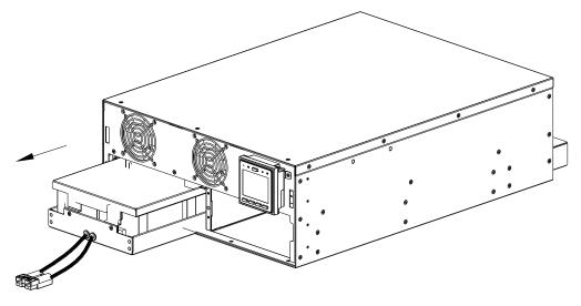
**7** Secure the brackets on UPS with 8 (M4x6) screws.
