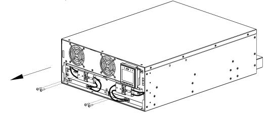
3 Disconnect UPS battery input wires.
