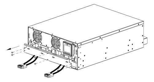
**6** Remove the battery modules from UPS.
