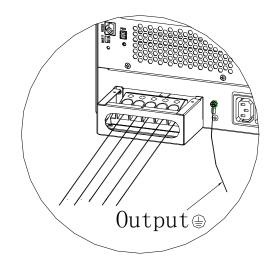
3 Connect the input wires to the first 3 terminals (counting from the left) and output wires to the last 2 terminals.
