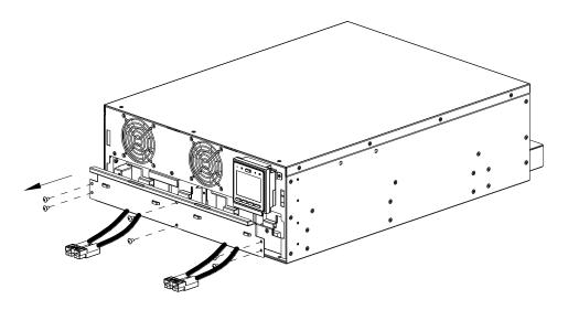
**5** Remove the battery modules from the UPS.
