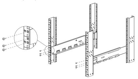
2 Secure the back of rail with 6 (M5x12) screws.
