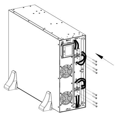
**11** Rotate the LCD of UPS 90 degrees to the right.
