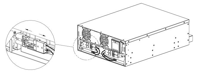
4 Remove the screws and the battery compartment door.
