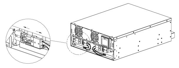
**5** Remove the screw and the battery compartment door.
