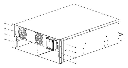
8 Rest the UPS on the rail. Slide the UPS into the rack.
