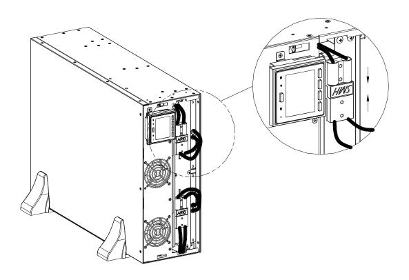
① Secure the battery connectors with 8 (M3x18) screws.
